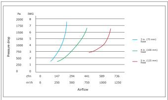
Please note that this pressure loss chart is an indication based on the combination of duct, rail and hose. For real values, please refer to hose documentation as well as mentioned hose diameter.
